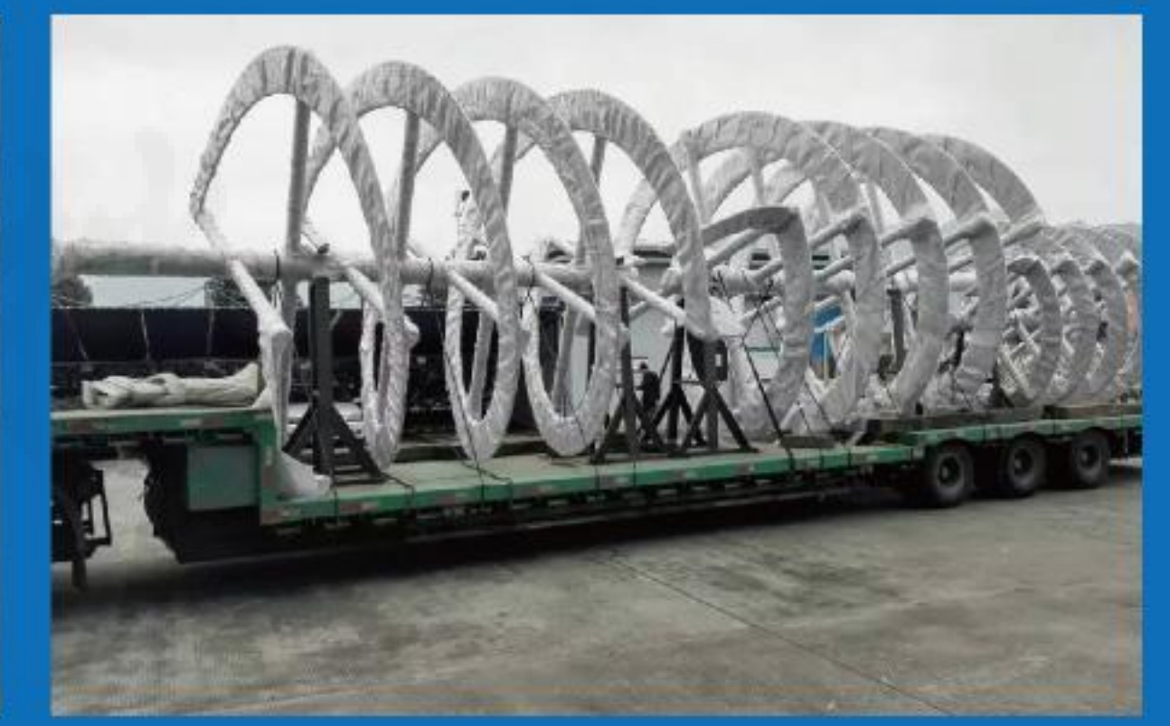
用于聚合釜的螺带式搅拌器 Helical Ribbon impellers (3.9m) for Polymerization Tanks
